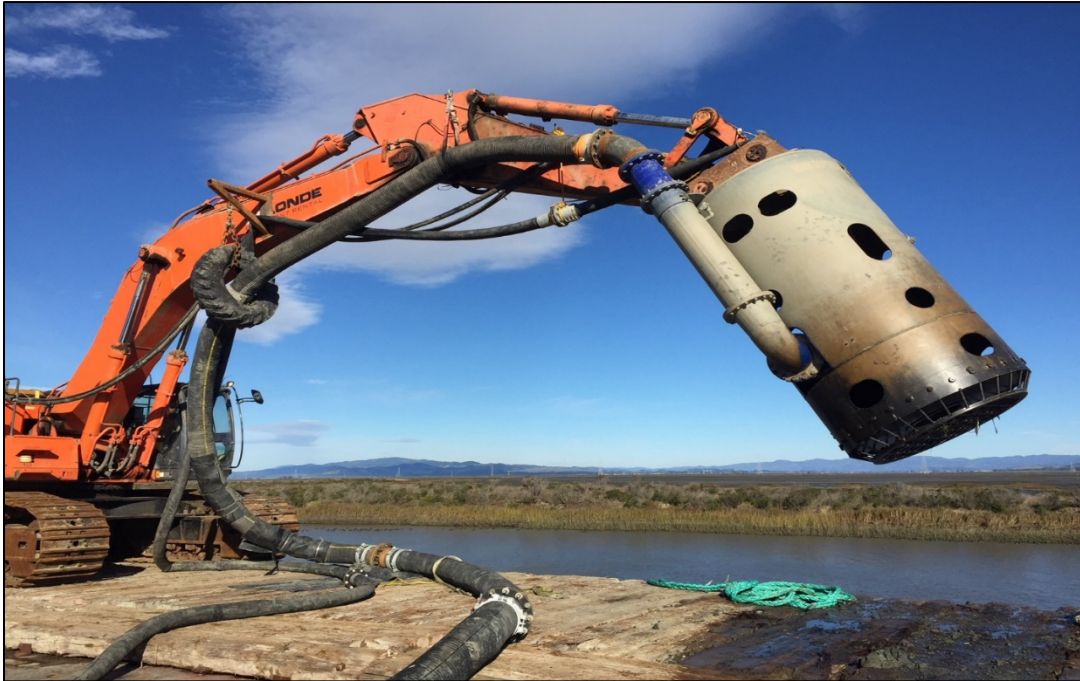
Figure 10: Modified Offloader Currently Offloading Dredged Material at Cullinan Ranch (Dutchman Slough)
